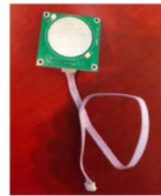
touch buttons + external cables (can be put under 3mm glass plate)
